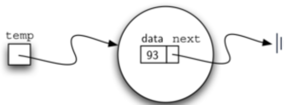
Figure 3.20: A Node Object Contains the Item and a Reference to the Next Node
